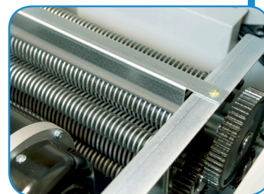
Solid steel gears, heat-treated cutting blades, AC geared motor
